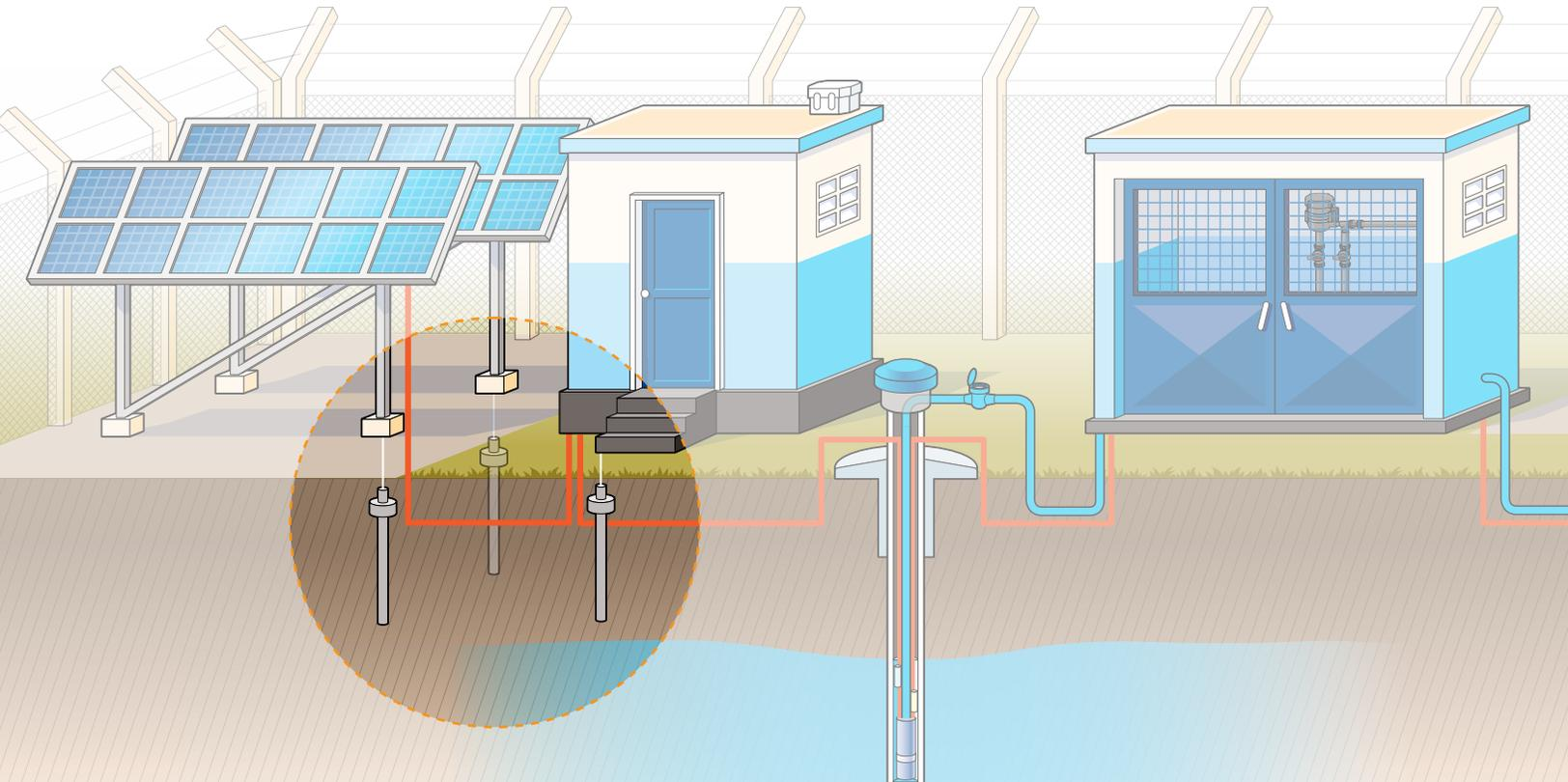
Grounding and electrical bonding protect against electric shock resulting from a conductor contacting exposed metal. Grounding is crucial for the safety of the people working around the system. However, grounding may have been overlooked in the design and installation phase.
