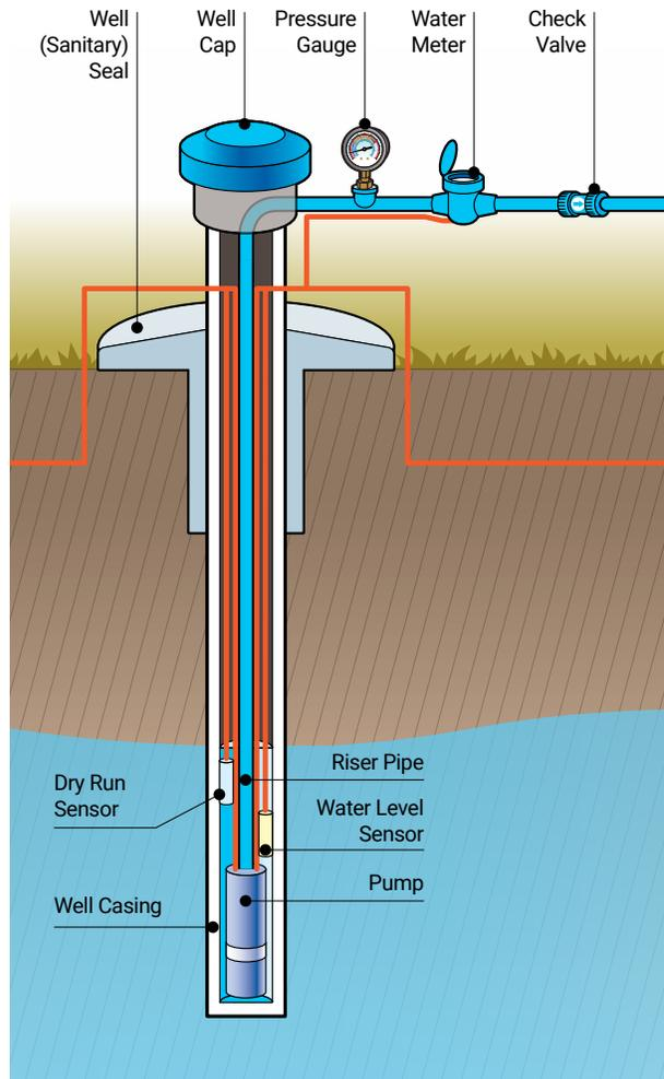
Most SPWS will have a submersible pump located within the well. If the well casing or riser pipe is metal, it is very important to correctly connect the pump wiring to the ground in the well casing.
