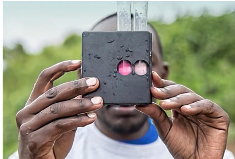
**Hach Chlorine Color Wheel test: Check the free and total chlorine and observe the System Operator performing the tests.**
